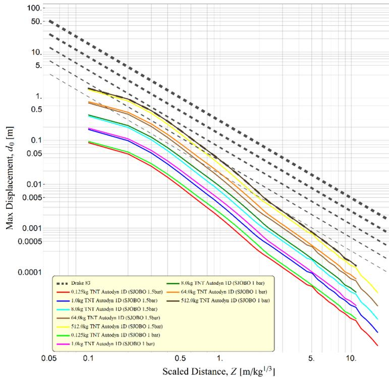
Figure 3: Maximum dry sand displacement  $d_0$  as a function of scaled distance  $Z$  for buried charges 0.125, 1, 8, 64, and 512 kg TNT for Drake 83 compared with AUTODYN.
