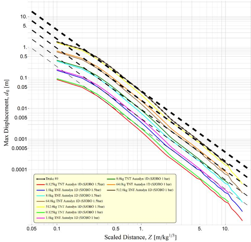
Figure 6: Maximum dry sand displacement  $d_0$  as a function of scaled distance  $Z$  for buried charges 0.125, 1, 8, 64, and 512 kg TNT using Modified scaling factor of 0.49 on Equation (5) for Drake 89 compared with AUTODYN.
