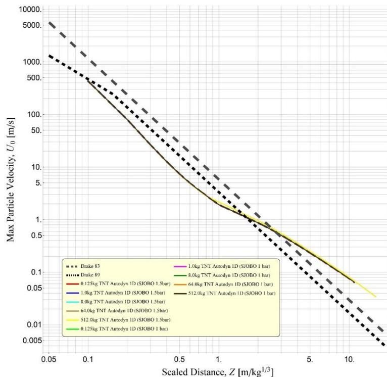
Figure 4: Maximum dry sand particle velocity  $u_{p0}$  as a function of scaled distance  $Z$  for buried charges 0.125, 1, 8, 64, and 512 kg TNT for Drake 83 and Drake 89, and 512 kg TNT for Drake 89 compared with AUTODYN.
