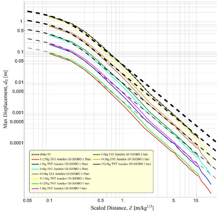
Figure 7: Maximum dry sand displacement  $d_0$  as a function of scaled distance  $Z$  for buried charges 0.125, 1, 8, 64, and 512 kg TNT Modified with saturation/tapering for smaller scaled distances  $Z$  by factor  $(1 - e^{(-30Z^{1.75})})$  and scaling factor 0.49 on equation (5) for Drake 89 compared with AUTODYN.
