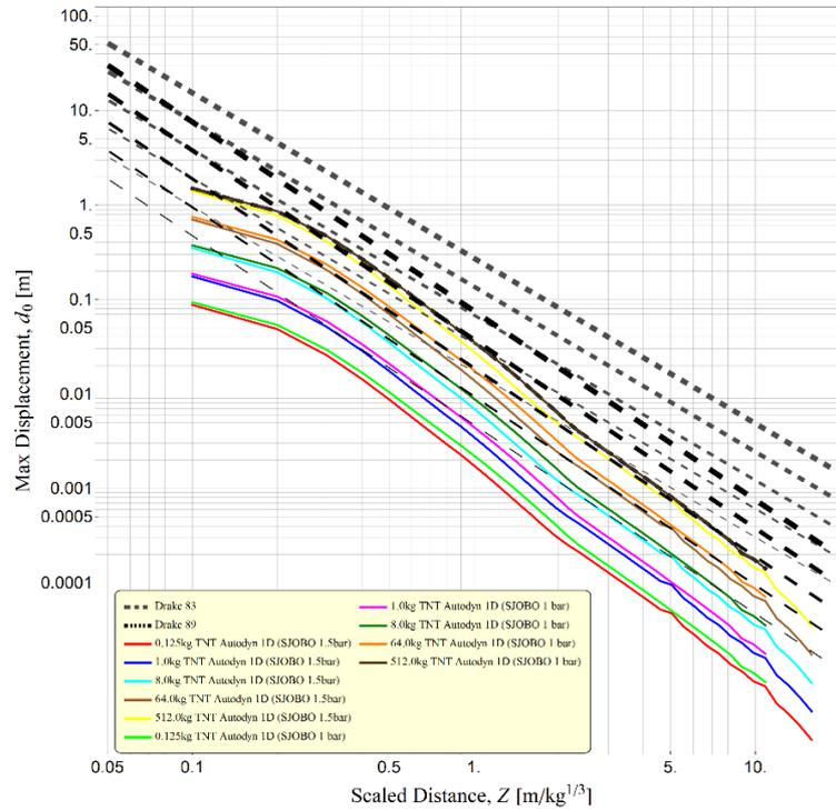
Figure 5: Maximum dry sand displacement  $d_0$  as a function of scaled distance  $Z$  for buried charges 0.125, 1, 5, 8, 10, and 125 kg TNT for Drake 83 and Drake 89 compared with AUTODYN.
